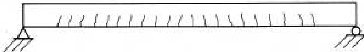
(c) Cracks where M \geq M_{cr}
